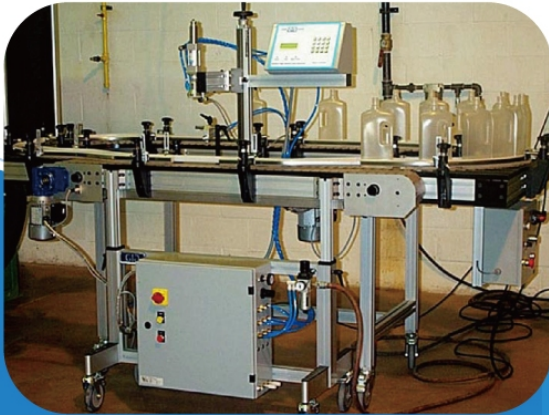
3 Leak Detector System
