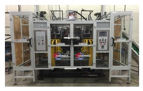
The Phoenix model 10-155F, shown above, is a state of the art extrusion blow molder with production scope as follows:
