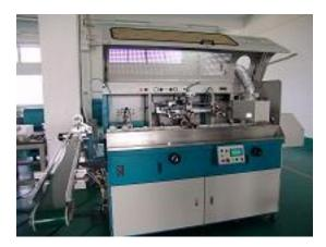
The S102 will automate the screen printing process for oval and cylindrical containers. It includes infeed conveyor (option available to upgrade to an automatic unscramble), flame pre-treatment, 1-color screen printing head with all the adjustments, UV curing station and automatic discharge to bulk or a conveyor.
